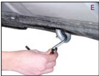
Attach S-hook to vehicle tow ring or other sturdy body part.
